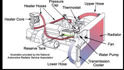
A heater core is a small radiator, located under the dashboard of the vehicle and consists of conductive aluminum or brass tubing with cooling fins to increase surface area. Hot coolant passing through the heater core gives off heat before returning to the engine cooling circuit.
